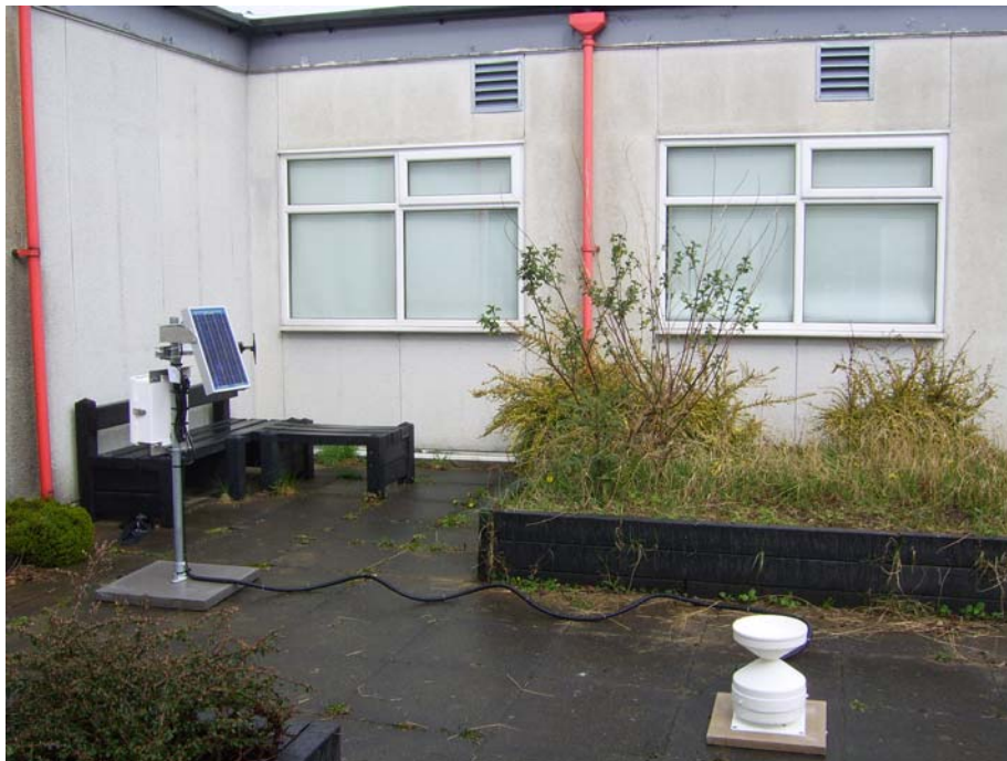
A newly installed rain-gauge at Middleton, Leeds
